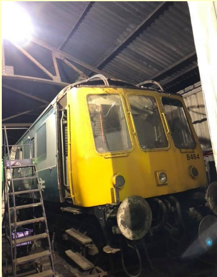
W51321 having cab tinworm attended to inside the shed at Shackerstone, 9/11/18 ( M.Miller )
